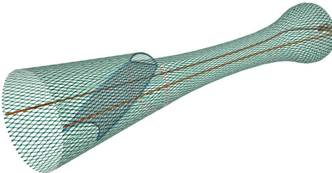
Figure 5. Inclined Separator Panel (Copyright 2004 reproduced with permission of FRS, Aberdeen).
