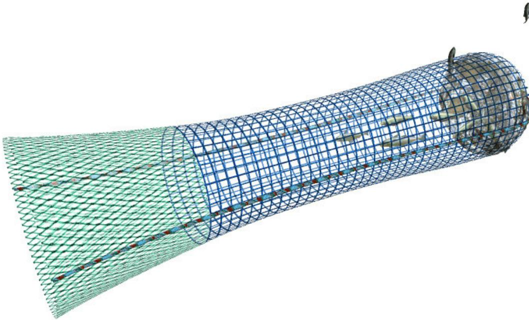
Figure 8. Full square mesh codend (Copyright 2004 reproduced with permission of FRS, Aberdeen).
