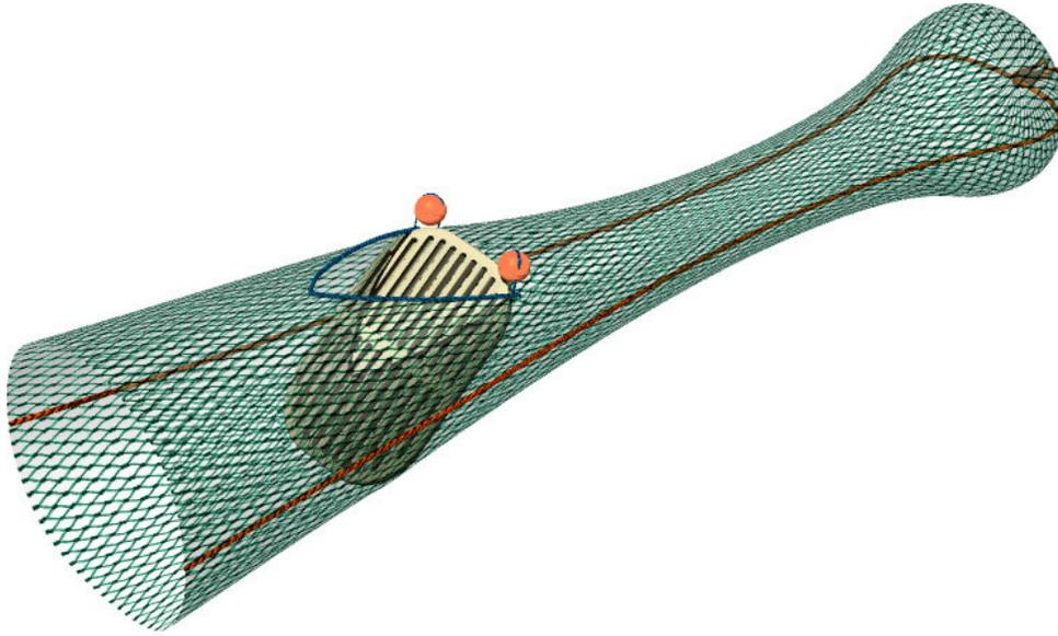
Figure 3. Nephrops trawl with grid (Copyright 2004 reproduced with permission of FRS, Aberdeen).
