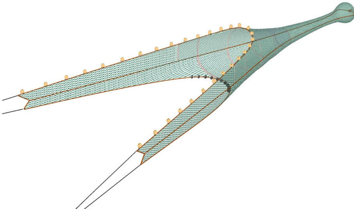
Figure 7. Cutaway trawl with set back headline (Copyright 2004 reproduced with permission of FRS, Aberdeen).
