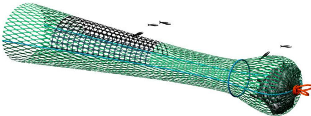
*Figure 6 Square mesh panel inserted in a diamond mesh codend (Copyright 2004 reproduced with permission of FRS, Aberdeen).*
